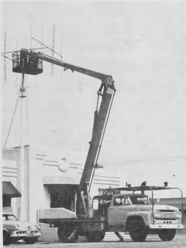
THE VERSATILITY of Lago's "giraffe" was displayed when the Marine Office antenna needed repair. E VERSATILIDAD di e "giraf" a worde demonstra ora e antena tabatin mester di mantencion.
